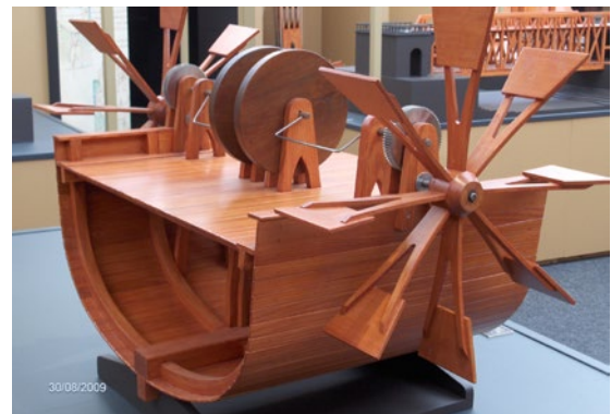
Principle of the paddlewheel boat
